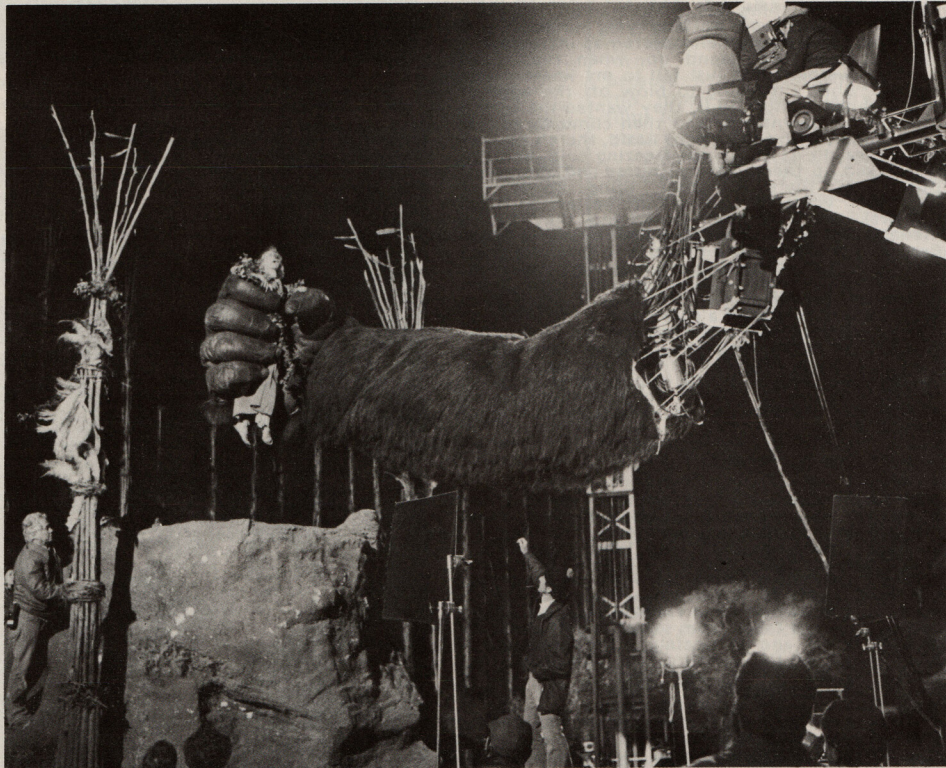
RIGHT: Kong's "stand-ins," the two hydraulically controlled hands which were used so extensively in the Paramount remake.
